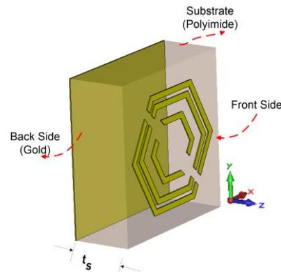
Fig. 1. Perspective view of the unit cell
