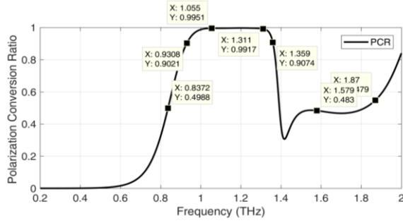
**Fig. 5.** Polarization conversion ratio of the proposed design.
