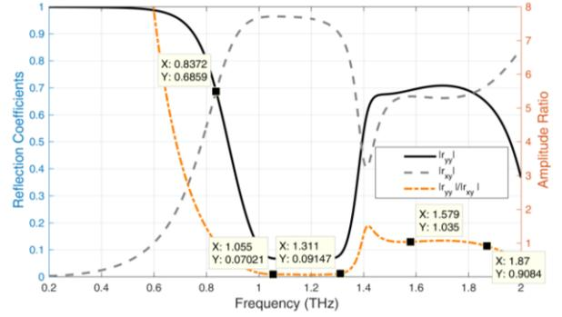
Fig. 3. Reflection coefficients (left) and amplitude ratio (right) of the proposed design.
