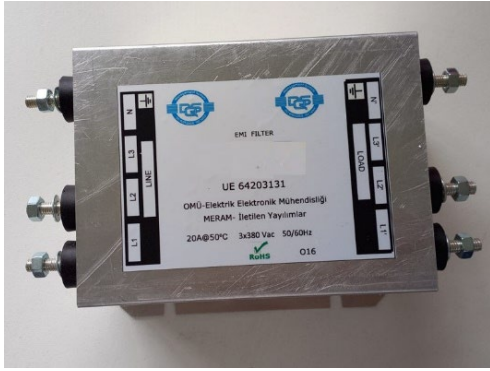
Fig. 6. EMI three phase filter application
