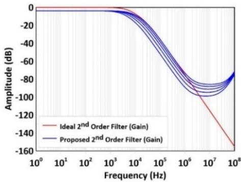
Fig. 8. 2<sup>nd</sup> Order Low Pass Filter Response With Regard To Different  $V_{SG}$
