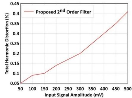
Fig. 10. THD Value With Regard To Input Signal
