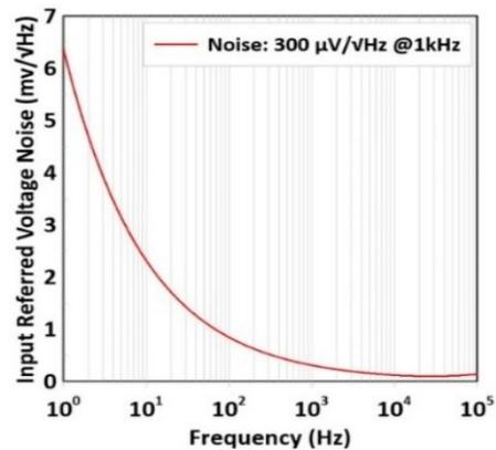
Fig. 11. Input referred noise behavior of the 2<sup>nd</sup> order filter
