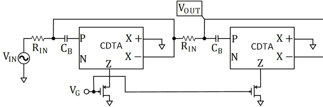
Fig. 7. 2<sup>nd</sup> Order Filter Structure Based On The Proposed Multiplier Circuit
