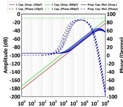
Fig. 5. Tunability And Multiplier Features Of The Proposed Circuit
