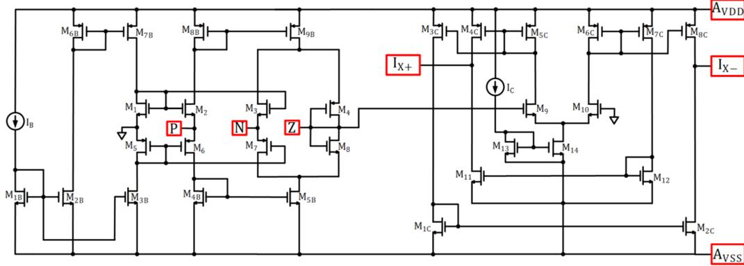
Fig. 4. CMOS Implementation Of CDTA
