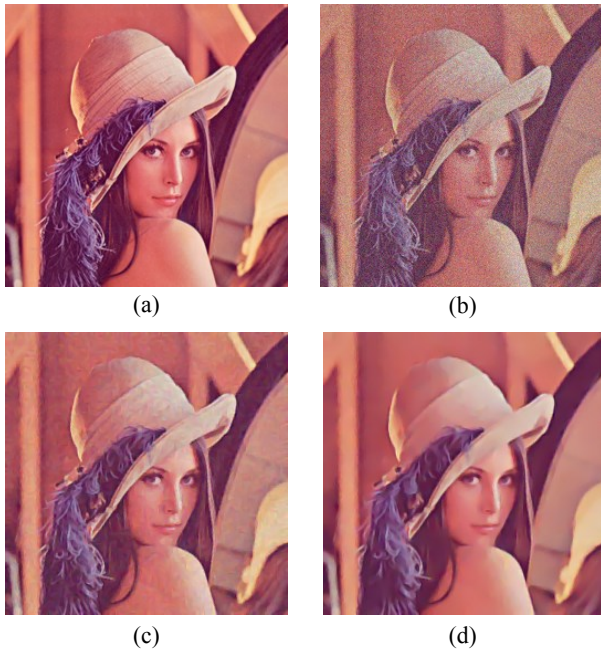
Fig. 4. Noise removal results for Lenna test image: a) Original image, b) corrupted image by Gaussian noise with \sigma = 20 and \mu = 0 , c) result of trace-based method (PSNR = 29.65 dB) [7], and d) result of presented method (PSNR = 30.40 dB)
