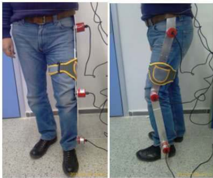
Fig. 3. The joint angle and foot force measurement system.
