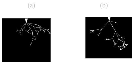
Fig. 8. Streamer patterns obtained for two values of the streamer conductivity (a) \sigma = 5 \Omega^{-1} \cdot \text{m}^{-1} (b) \sigma = 50 \Omega^{-1} \cdot \text{m}^{-1}
