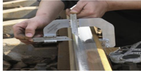
Fig. 1. Manual rail measurement [7]
