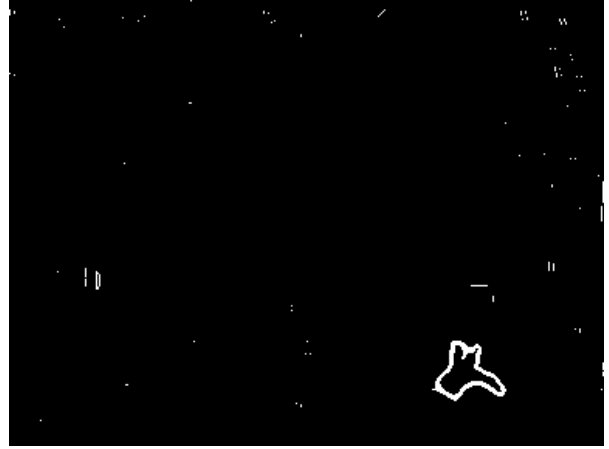
Figure 3. Contour map differences between background model (Fig. 2) and frame no. 180 from Walk3 sequence
