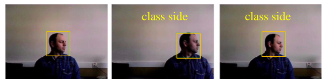
Fig. 1. Tracking results obtained by the color based particle filtering on video frames including self-occlusion.
