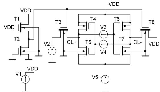
Fig. 2. Circuit for SNM simulation and measuring
