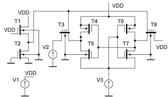
Fig. 4. Circuit for discharge current simulation and measuring
