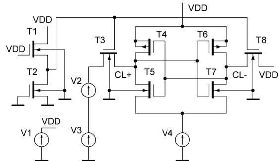
Fig. 3. Circuit for WRM simulation and measuring
