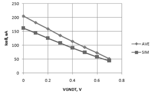
Fig. 10. Dependency of  $I_{cell}$  on the potential of the supply bus of the trigger
