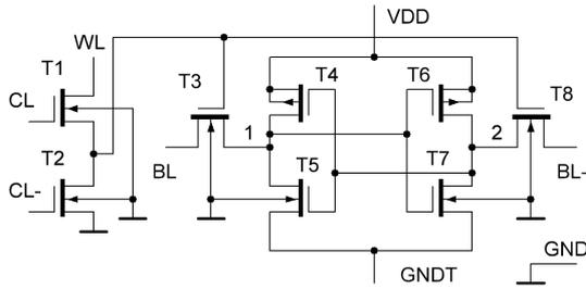
Fig. 1. Circuit of the proposed memory cell
