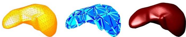
Figure 5. SOFA architecture of an object; left to right: collision, behavior and virtual models
