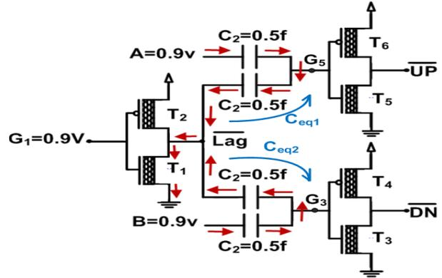
Fig. 4. The discharge paths of the  $\overline{Lag}$  node, which are shown with red vectors
