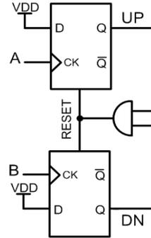
Fig. 1. Logic schematic of the conventional PD
