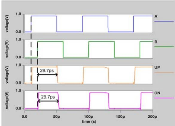
Fig. 6. The waveforms of the designed PD for an input frequency of 12.5GHz and the two inputs are  $45^\circ$  out of phase.
