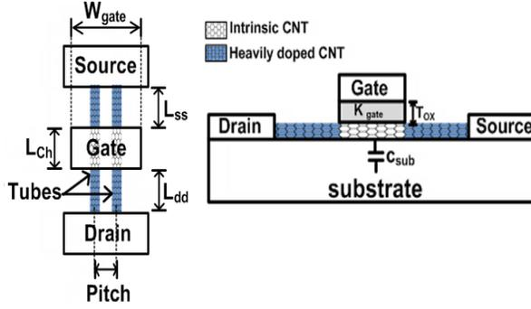
Fig. 5. Presentation of modeled CNFETs and relevant parameters
