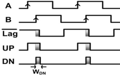
Fig. 3. The waveforms of the proposed PD
