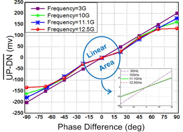
Fig. 7. I/O characteristics of the proposed PD
