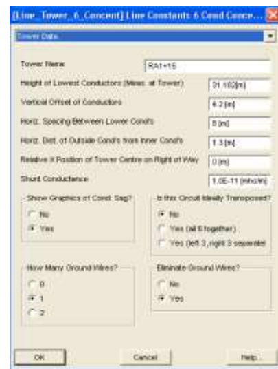
Fig. 7. RA1+15 tower main part dimensions
