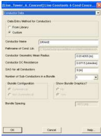
Fig. 8. 795 MCM Drake conductor data
