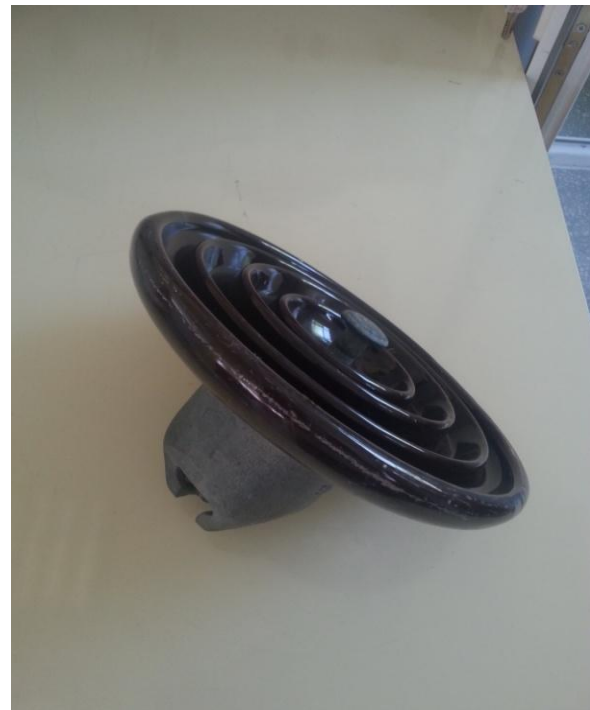
Figure 4. Photograph of U160 BL Insulator
