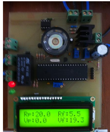
Fig. 3. The developed electronic control card for a sustainable power management
